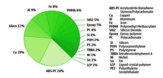
Figure 2 Material composition of a mobile phone circa 2006.<sup>34</sup>
