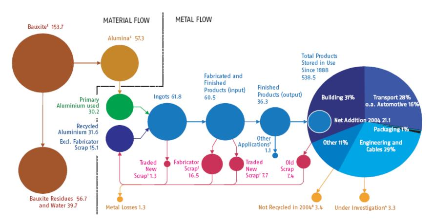
Values in millions of metric tonnes. Values might not add up due to rounding. Production stock not shown.
