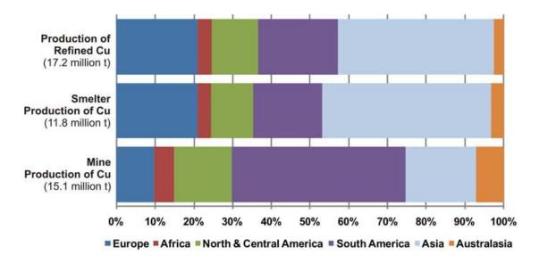
Figure 12 Global distribution of mined, smelted and refined copper in 2006.<sup>129</sup>
